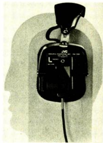
FIG. 4—JVC MODEL HM-200E contains microphone and baffle combination with characteristics that approximate the human ear.
